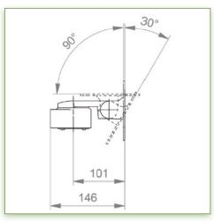
Display Compatibility: 26" Wide ( Weight) Supported Weight: 20 Kg VESA standard: 75 / 100 mm Keyboard-Mouse holder: 485 x 220 mm
