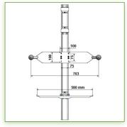
Display Compatibility: 26" Wide ( Weight) Supported Weight: 20 Kg VESA standard: 75 / 100 mm Keyboard-Mouse holder: 580 x 200 mm
