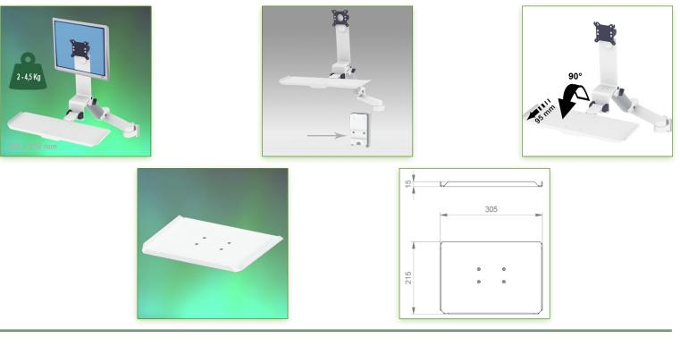
Display Compatibility: 26" Wide ( Weight) Supported Weight: 2- 4,5 Kg VESA standard: 75 / 100 mm Keyboard-Mouse holder: 300 x 210 mm
