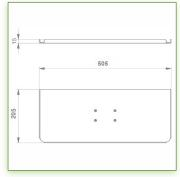
Display Compatibility: 26" Wide ( Weight) Supported Weight: 13 - 16,5 Kg VESA standard: 75 / 100 mm Keyboard-Mouse holder: 500 x 200 mm
