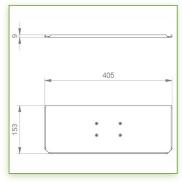
Display Compatibility: 26" Wide ( Weight) Supported Weight: 13 - 16,5 Kg VESA standard: 75 / 100 mm Keyboard-Mouse holder: 400 x 150 mm
