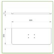
Display Compatibility: 26" Wide ( Weight) Supported Weight: 11 - 12,5 Kg VESA standard: 75 / 100 mm Keyboard-Mouse holder: 500 x 200 mm
