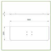
Display Compatibility: 26" Wide ( Weight) Supported Weight: 6 - 10,5 Kg VESA standard: 75 / 100 mm Keyboard-Mouse holder: 580 x 200 mm
