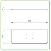
Display Compatibility: 26" Wide ( Weight) Supported Weight: 3 - 8 Kg VESA standard: 75 / 100 mm Keyboard-Mouse holder: 400 x 150 mm
