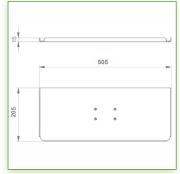
Display Compatibility: 26" Wide ( Weight) Supported Weight: 13 - 16,5 Kg VESA standard: 75 / 100 mm Keyboard-Mouse holder: 500 x 200 mm
