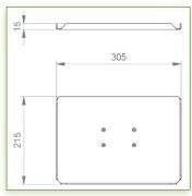
Display Compatibility: 26" Wide ( Weight) Supported Weight: 13 - 16,5 Kg VESA standard: 75 / 100 mm Keyboard-Mouse holder: 300 x 210 mm
