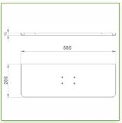
Display Compatibility: 26" Wide ( Weight) Supported Weight: 2-5 Kg VESA standard: 75 / 100 mm Keyboard-Mouse holder: 580 x 200 mm
