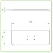
Display Compatibility: 26" Wide ( Weight) Supported Weight: 2-5 Kg VESA standard: 75 / 100 mm Keyboard-Mouse holder: 400 x 150 mm
