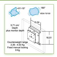
Display Compatibility: 26" Wide ( Weight) Supported Weight: 2,26 - 9 Kg VESA standard: 75 / 100 mm
