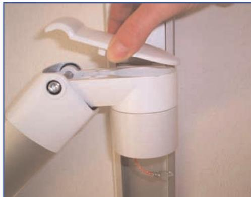
8. Remove the right hex screw M 6 x 12 and replace it with the hex key M 6 x 40. Fasten the screw until the depth gauge without using any force.
