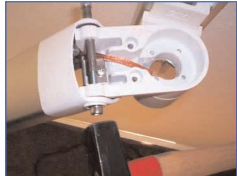
9. Lead the spiral cable wrap with the cables from below through the console and from above through the inner pivot block into the support arm profile. Lead the spiral cable wrap from the support arm profile downwards through the outer pivot block
