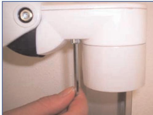
7. Disengage the locking lever and bring the arm in position may the inner cover be removed.
