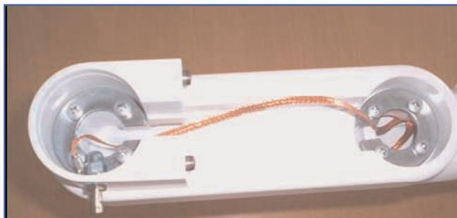
3. Remove the end caps and the aluminium profile (if not removed already).
